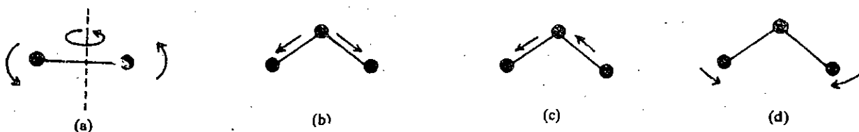
Fig. 7.1 : Rotation and vibration within molecules: (a) shows rotation about two different axes; (b), (c), and (d) show vibrations. (b) and (c) are referred to as stretching and (d) as bending.
