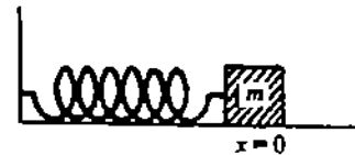
Fig. 8.9: Mass on a spring as a one-dimensional harmonic oscillator.
